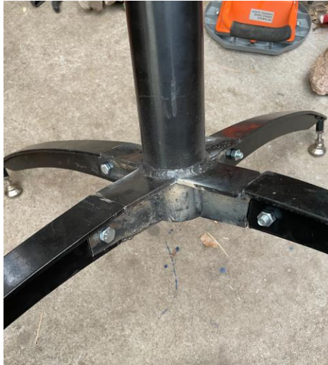
Figure 4: Stand Column and Legs Bolt Arrangement
